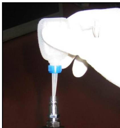
Figure 9 – Lubricating the nozzle.
