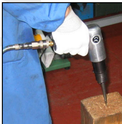
Figure 8 – Starting the air hammer.
