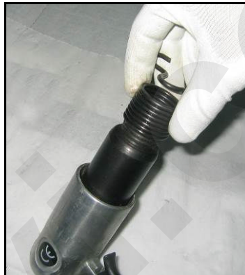
Figure 5 – Removing the lock.
